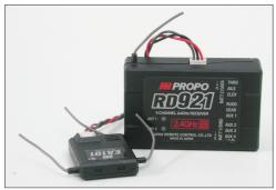
The JR RD921 receiver features two types of fail-safe: SmartSafe and Preset Fail-Safe.
