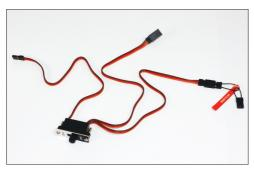
2. Turn on the receiver switch. Note that the LED's on all receivers should be flashing, indicating that the receiver is ready to bind.
