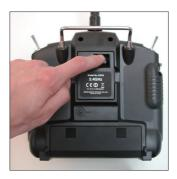
5. Remove the bind plug from the receiver or switch harness and store it in a convient place.
