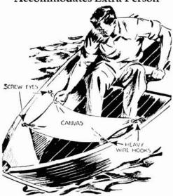
This boat seat, which is made from heavy canvas, comes in handy when carrying an extra passenger. It hooks into screw eyes driven into the boat sides and is quickly removed and rolled up when not in use.
