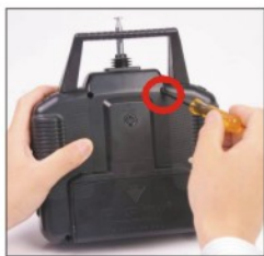
1. 打开背后四个螺丝 Open the rear four screws.
