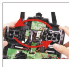
10. 取下一四通道后的操纵杆组对换 exchange the operating rod sets without the first and fourth channels.
