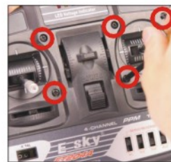
5. 取下左右操纵杆 四个螺丝 Unload the four screws of
