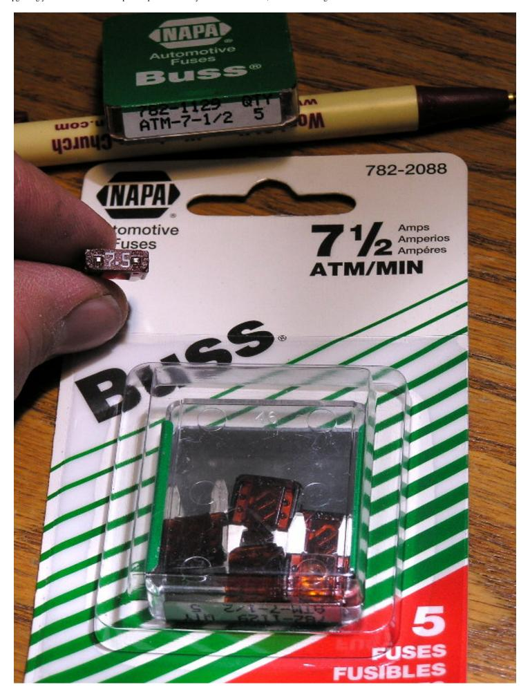
The photo above is an example of the fuses. The fuses you need are the <u>small mini-Blade</u> <u>automotive fuses</u> available at any automotive parts store. Use the mini-blade fuses as they are smaller and lighter than the normal blade fuses (weigh less than .5 grams). Use 7.5 amp for the main motor and 2 (preferred) or 3 Amp for the tail motor.
