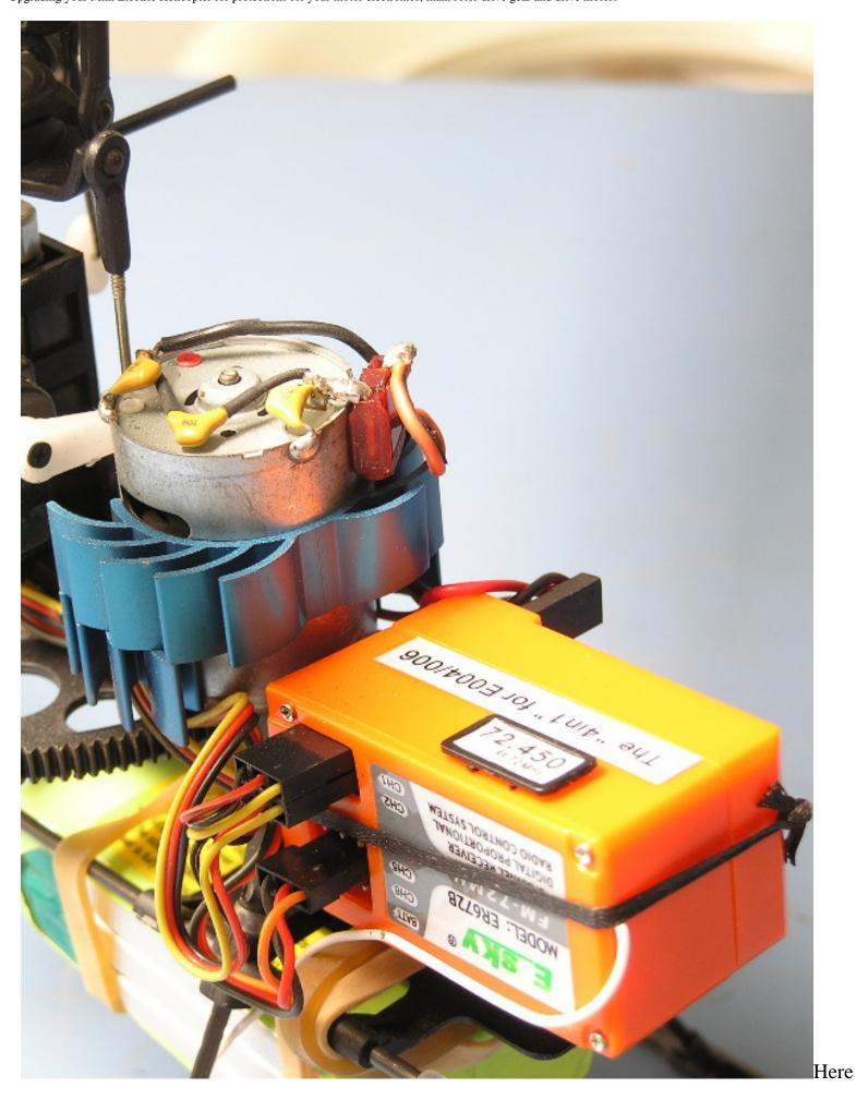
is another view from the other side of how to mount your 7.5 amp fuse. (Normal power draw when the helicopter is in flight is 3.5 - 5.5 Amps so the fuse will never blow unless you hit something) If you do hit something you want the motor to stop immediately as you are going to do less damage to the rotor system if it is not under power when it bumps around hitting things on the way to the ground.
