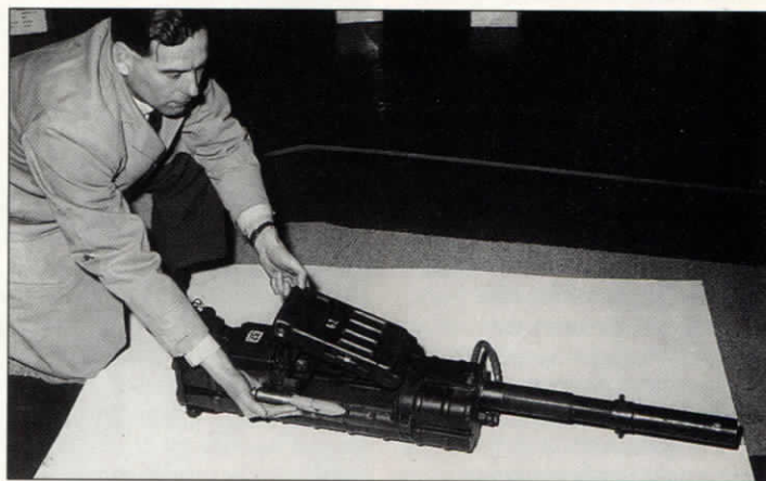
ABOVE The Rheinmetall-Borsig MK108 30mm cannon. A technician holds one of the 330g (11oz) high-explosive rounds. BELOW An Me 262A-1a of JG7 with 12 R4M 55mm folding-fin rockets mounted on a wooden rack under the starboard wing.
