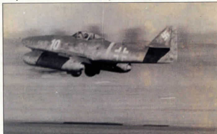
ABOVE Me 262A-1a "White 10" of Ekdo 262 takes off from Lechfeld. The undercarriage was retracted early to reach the single-engine safety speed of 180 m.p.h. as soon as possible.
