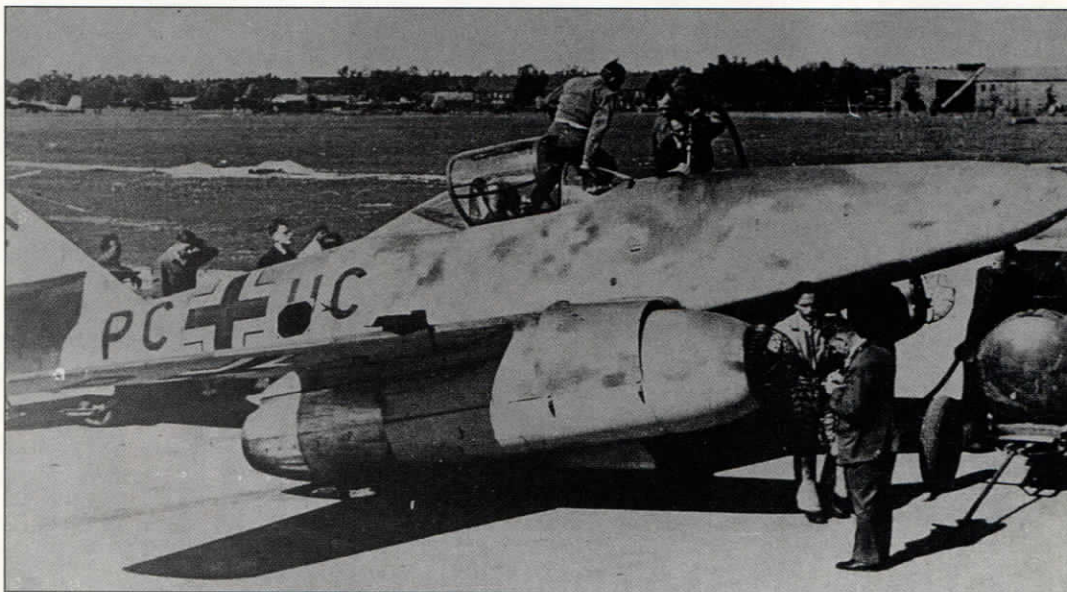
ABOVE The V3 prototype, PC+UC, was the first Me 262 to fly on jet power alone, on July 18, 1942. The early Me 262 prototypes were fitted with a tailwheel undercarriage arrangement.
