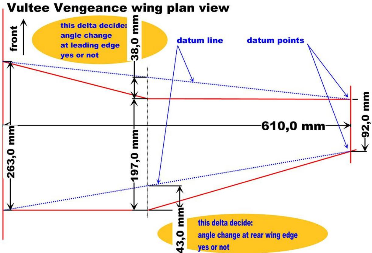
You can see clearly that there is more than 20mm deviation from the datum lines (-----) at both the leading and trailing edges of the wing. This means your model should also be built with this angle change.
