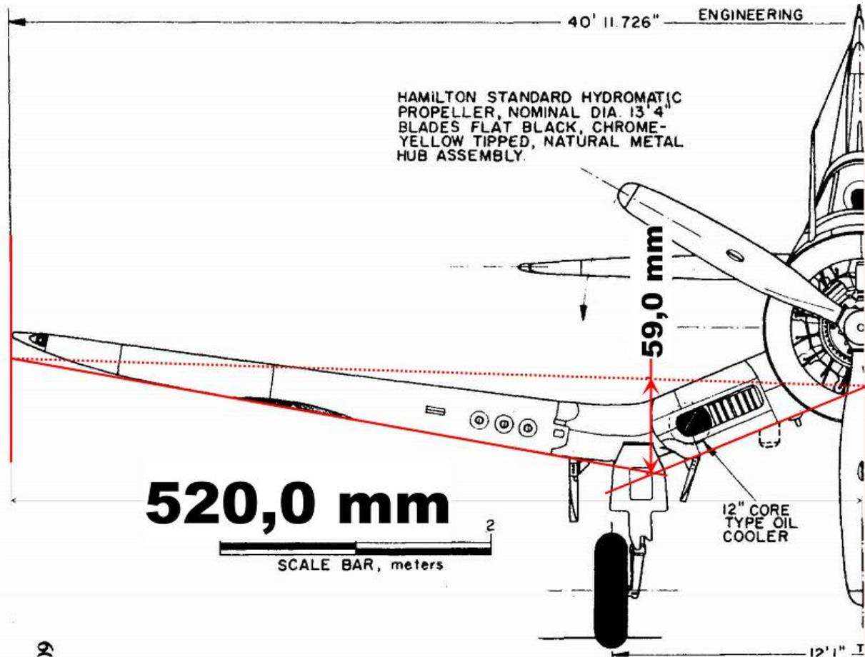
If we look at the drawing of an F4U Corsair, you can see the difference between the datum line (-----) and the bottom surface of the wing is more than the allowed 20mm deviation. In this instance you can see your model wing will need to be built with a crank/angle change to remain within the 20mm permitted tolerance.
