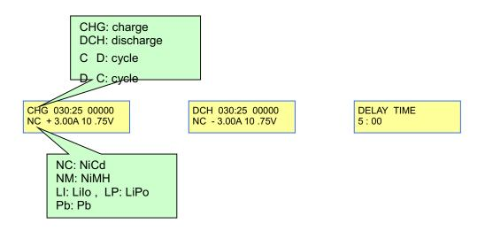
If the Enter button is pressed, charge or discharge can be finished.
