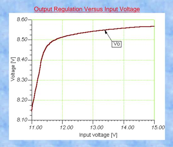
The above graph shows how the output is affected by input voltage variations. This was produced with a load current of 100mA and using a 10 volt rated zener diode. Note that the circuit falls sharply out of regulation when the input voltage falls to 11.5 volt, hence the requirement for an adequate supply voltage.
