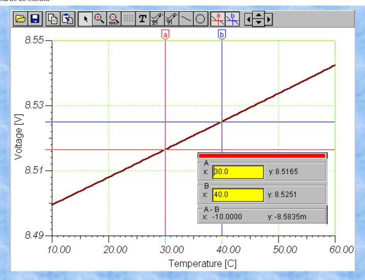
Temperature stability is very good as the above graph shows. The output voltage changes by 8.5mV for every 10 degree rise in temperature. This is less than 1 mV / degree.
