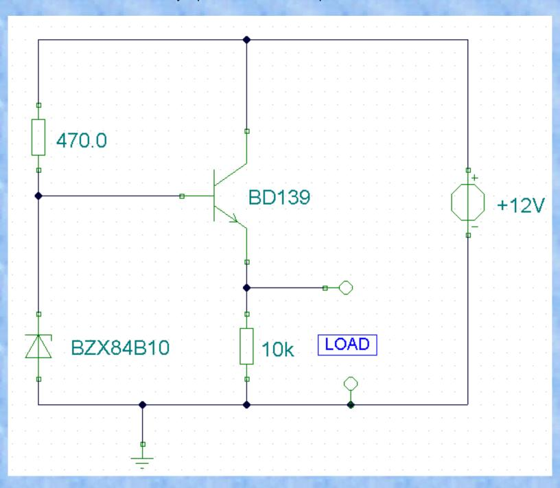
The output voltage is equal to the zener diode voltage less 0.7 volts, or :-
