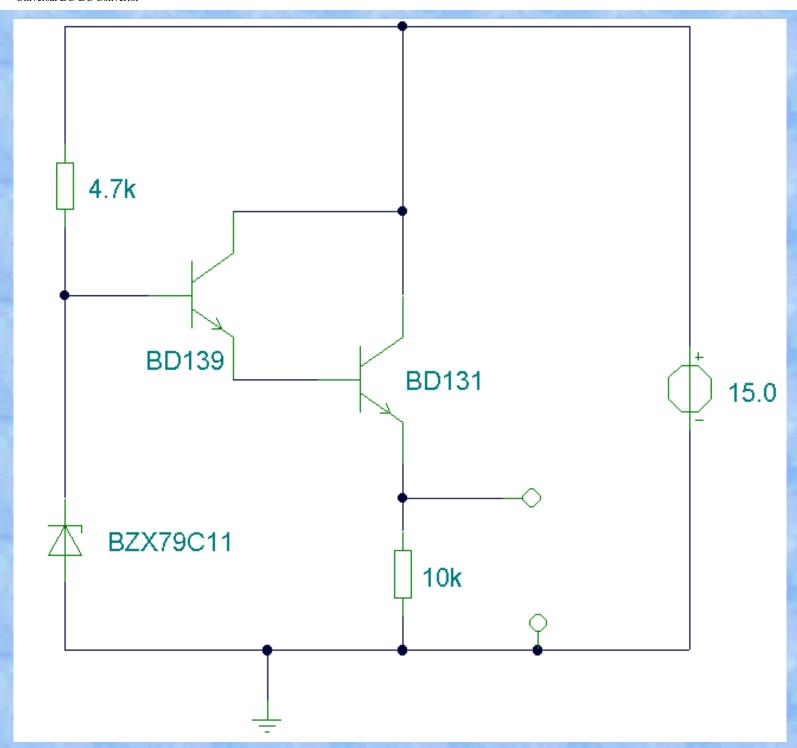
Output dissipation is calculated in the same way, the BD131 has a maximum power dissipation of 15 watts and collector current of 3 amps. The output voltage is approximately 1.4 volts less than the zener diode voltage and supply voltage must be higher than the input voltage by at least 3 volts.
