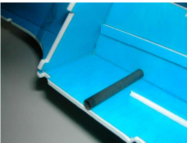
2) Fix the reinforce carbon tube
