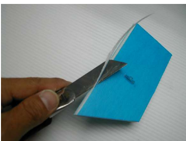
15) Use a knife to cut the control surface at an 45 degrees angle
