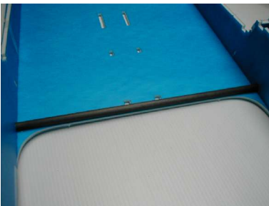
4) Reinforce Carbon tube between left and right hull
