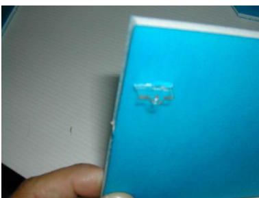
14) Use epoxy to glue the control in all control surface
