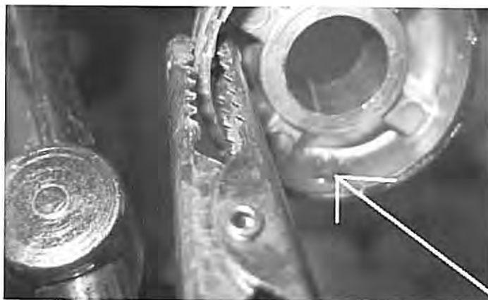
This view shows the actuator magnet, epoxied into a hole drilled in the engine thrust washer. This needs to be very secure, so the magnet doesn't become an airborne projectile.
