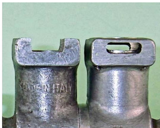
Barbini B.38 - production (L) and prototype (R) cases
