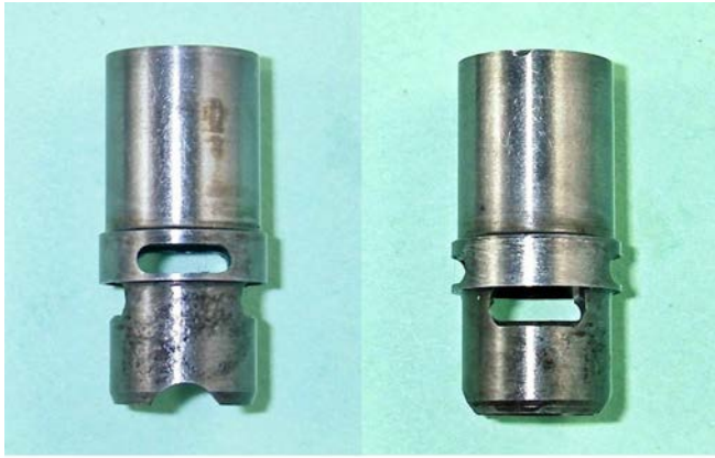
Barbini B.38 cylinder showing porting - exhaust L, transfer R
