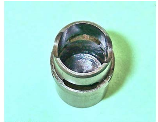
Barbini B.38 cylinder showing transfer port chamfer
