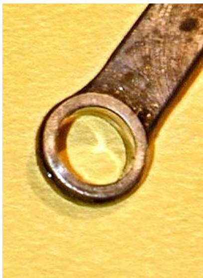
Barbini B.40 needle roller big end (Ron Chernich)
