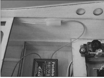
☐ 7. We used small scraps of fuel tubing we had laying around the shop and glued them to the sides of the fuselage to support the antennas of the 2.4GHz receiver shown in the picture. If you are using an FM or PCM receiver, an antenna tube is provided between the two outer pushrod tubes.
