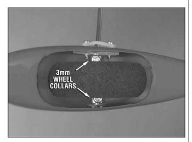
□ 6. Install a 3x4mm machine screw with threadlocking compound in two 3mm wheel collars. Remove one of the screws from the landing gear strap and install on the landing gear a wheel collar, wheel and a second wheel collar. Insert the landing gear in the wheel pant retainer and reinstall the landing gear strap. Tighten the 3x4mm machine screws in the two wheel collars. Make sure that the wheel rotates freely. Repeat this step for the other side.
