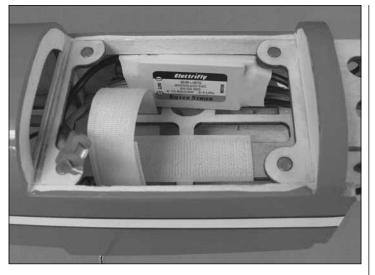
□ 5. Cut a piece from the included double-sided foam mounting tape and attach the ESC to the side of the battery compartment. Connect the ESC to the motor. Now would be a good time to use your radio system and battery to confirm that the motor rotates in the correct direction. If the motor does not rotate counter-clockwise when viewing it from the front, simply disconnect any two of the three motor leads and swap their positions.
