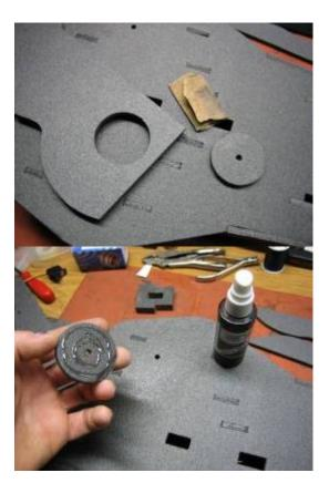
5. Build the wings next... Sandwich the .030  $\times$  .236 carbon spar between the two foam pieces. It's easiest to glue all three parts at the same time. Make sure the carbon is flush with the foam.
