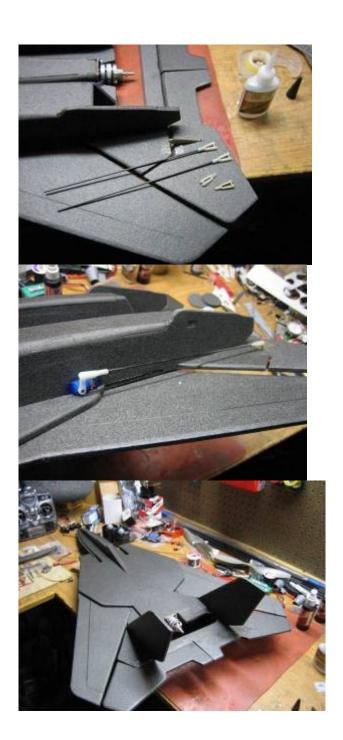
13. It's just not an F-14 without the deck ribs... I used some 2mm depron I had laying around. The ribs also add stiffness to the upper deck.
