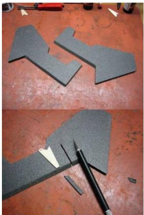
12. I use tape hinges because they are quick and easy but other hinge methods work well too. Tape both sides and add additional perpendicular strips at the ends to prevent the tape from tearing.
