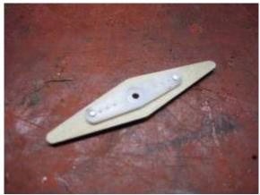
7. Some packing tape let's the wing slide smoothly against the lower deck. The rear spacer, pivot disc and forwards spacers are all load-carrying parts when glued so be sure not to put tape near any of these parts.
