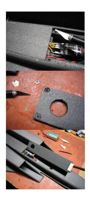
4. Flip 'er over and build the top side now... lightly sand the inside of the wings to fit the pivot discs if needed
