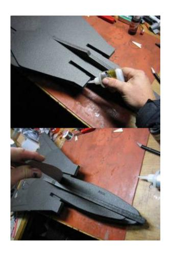
11. Install the rear deck, motor mount and motor. I use CA for the motor mount with good results, but epoxy will be stronger. Chamfer the TE of the deck to match.
