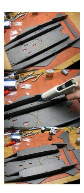
2. Fuselage is next... watch out for the engine mount tabs that protrude out of the top side. Glue the doublers in next. Align the kink in the doubler with the deck joint. Temporarily install the hatch and rear bottom piece and position the inlet piece. Chamfer the inside edge of the inlet LE so that it form scoop. Glue the inlet piece only at this time.
