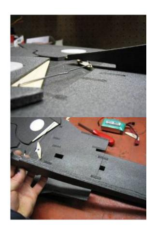
9. Glue the fwd spacers in - remember that these parts carry some of the wing loading so apply glue near the edge.
