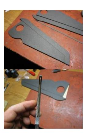
6. Assemble the wing servo arm using a couple of servo mounting screws, then cut and grind the screws
