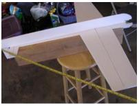
In the area indicated in shade, Install 3/4" strapping tape on both sides of the fuselage. Trim it as shown for a taper from 10" to zero at the stabilizer trailing edge. Use a heat gun or hair drier on low or a covering iron with a cover sock to adhere the tape to the fuse. Do not overheat the foam. It is more resistant to heat than most foam but can be melted.
