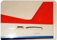
Use your fingers to locate the pre-cut openings underneath the covering. Then use a sharp hobby knife to remove the covering as needed. Becareful not to cut into any surrounding wood surfaces during this pricess.
