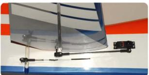
Locate the pre-slotted elevator servo tray in the tail along the right side of the fuselage. If you haven't done so already, use a sharp hobby knife and remove the covering over the servo tray.
