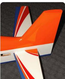
Remove the horizontal stabilizer from the fuselage to reveal your cou marks.
