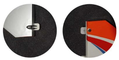
If the hinges do not slide in freely, open up the slits a little bit using a hobby knife.
