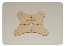
Right thrust has already been incorporated into the engine mount.
