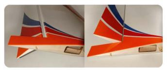
Once you have attach CA hinges to both ailerons, slide them into position onto both wings.
