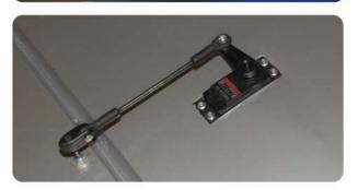
Locate the pre-slotted aileron servo trays on the bottom surface of both main wing panels.
