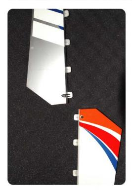
Notice that each elevator half has 4CA hinge slits with corresponding hinges slits on the horizontal stab pre-cut at the factory.
