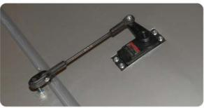
With the pushrod connect to the ball linkage center the servo arm and aileron again.
