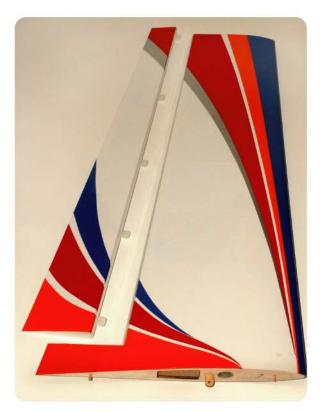
Each aileron is pre-slotted and equipped with four CA hinges. Slide the hinges in halfway in the position shown above then attach them using thin CA glue.
