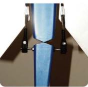
Insert the torque rod into the opening you made on the rudder.
