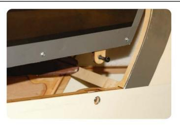
At this time, remove the hatch from the fuselage and notice the two screw holes on the side of the hatch.
