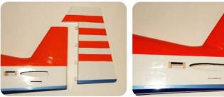
Locate the four hinges slits on the rudder and slide the CA hinges in halfway. Use thin CA glue to securely attach them.
