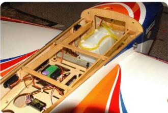
As shown in the top picture. When you use over size power source with model, we are recommended make a reinforcement with additional contained parts.
