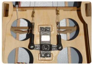
Locatie the pre-slotted pull/pull servo tray inside the hatch. It is currently slotted for the hitec HS-654MG servo.
