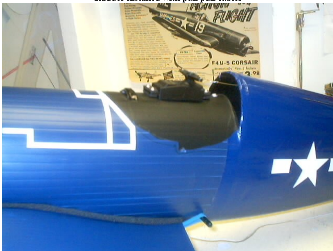
Rudder installed with pull pull cables
