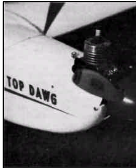
Note flexible loop on OS Max .10 to allow for servo overtravel.
