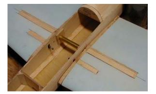
Internal reinforcing plates can go on the brass tube. I drilled 9MM holes in them over wood backing & sized them to not interfere with cam motion. With panels aligned, the plates were slid inward to coat with epoxy. When cured, remove the panels & fill the gaps around the tube ends.
