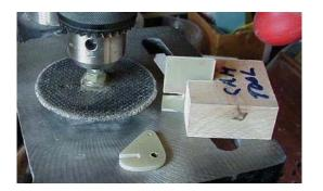
Cams are to have holes on 5/8" centers as plans show. 2-56 ball links will self tap into a 3/64" hole. For 1/8" pivot wire, use #30 bit. Optionally, a piece of 5/32" brass tube can be seated in a 5/32" hole. Use disc sander to shape as plans show. Cams in Harley's package are slotted rectangular pieces.
