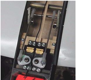
Here JR micro digitals were installed. Output arms need to be sturdy, so wheels are used & trimmed for clearance.
