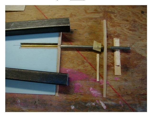
A rise of 1/16" over 3-1/2" is one degree. Add 1/16" to the shim. At a point 3-1/2" from the cap, mark on masking tape. Place the shim there to angle the tube down in the panel. The outer ends of the tubes should not protrude from the cores. Run a thin bead of quick epoxy along the tube & facings, avoiding the ends where the rod or endcap may get bonded. Using the shim, repeat the procedure on the other panel. Remove & set the endcaps aside for now.
