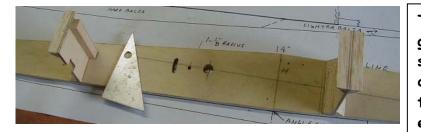
To the front of F1 & both sides of F2, glue triangular stock (TS) so all is squared up to the sides. With a side down flat, glue formers to it. To glue to the other side, position sides upright with everything squared up.
