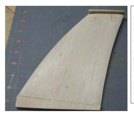
After mostly shaping the fuselage, clamp the fin blank between the sides, flush along the bottom. 1/8" above the sides, mark fillet lines. Remove fin. Along LE & TE, mark centered reference lines.
