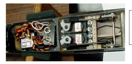
Jay Decker used the 150 oz./in. Hitec HS 5945 servos and Rocket City Missing Link type fittings. Servos were lowered to lower the pushrods up front.
