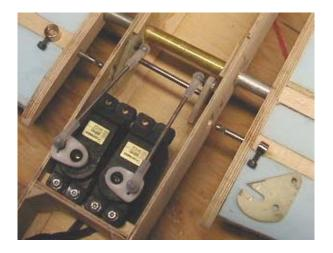
Panels, fitted with tubes, rotate on a 5/16" steel rod. 1/8" drive pins, notched for wheel collars, protrude to enter a slot in a cam (lower right). Cams pivot on a 1/8" shaft across the fuselage. Cams, shimmed with washers to clear the sides, are fitted with 2-56 threaded ball links, same as the servo output arms. Pushrods are all-thread 2-56 steel wire. At the rear, as shown in the next picture, servos mount to a 1/8" ply crosspiece secured to rails.
