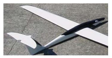
The '07 version has equal sweep along the LE & TE. The pivot point is located at 45% of chord. This aerodynamic balancing makes less work for the servos.
