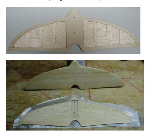
An easy way to apply glass is to lay down a piece, smooth it out, lightly spray a stab surface with 3M77, etc. Then press the stab to the glass. Apply a little instant CA glue along the perimeter to seal the glass there. Sand off excess glass, coat the one surface with bagging epoxy & roll with toilet tissue to sop up the excess. Let it cure. Repeat on the other surface. When cured, sand smooth, apply the "slurry" mentioned in File 1, pg.16, to prime & paint. This stab weighs approx. 1.5 oz.
