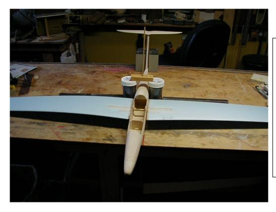
Weights (dry battery cells & lead shot in jars) were used to keep the fuselage upright & centered over its line. The tips of the cores were also weighted down flat to the bench to stabilize things. The block with the dowel in it is used to check alignment of fin to fuselage.
