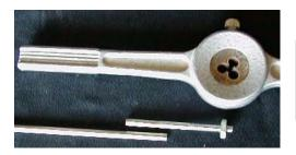
A piece of 1/8" stainless steel welding rod can easily be partially threaded with a 6-32 die. Clamp it upright in a bench vise to make threads. Notch the smooth end.
