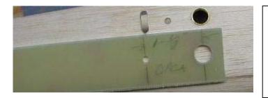
From 1/8" ply, epoxy board, etc. drill 11/32" & 5/32" holes on 1-1/8" centers. From the 11/32" tubing, cut off a piece 5/8" long. Smooth an end & run it through the stacked sides with some protruding (not shown here) to drill a series of 1/8" holes in an arc pattern.
