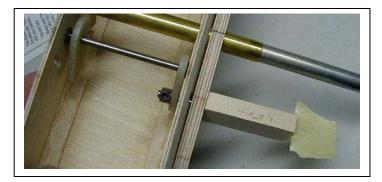
To get all clearances just right, seat the 2-56 ball links in the cams. Slide the 1/8" pivot wire through one side, slip on washers for clearance, then both cams & the other washers. Slide the pivot wire into the other side. Rotate the notch so the setscrew will be accessible. Run a stud into the collar as a handle to easily screw the threaded pin into the block. Determine how much of it should protrude to eliminate play between a panel and the fuselage. Take a measurement to the center of the
