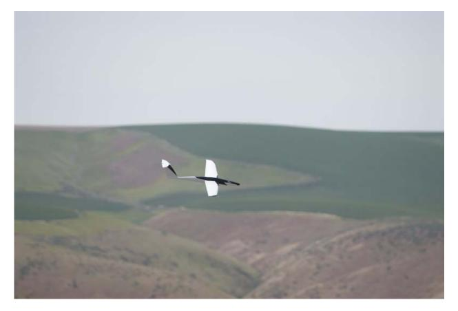
Employing a Tx with <u>elevon</u> function, panels rotate in opposite directions for turn & in the same direction for pitch to provide solid, stable, smooth, coordinated maneuvering. See setup & flying comments, pg.14. With Rx, servos, 4 cell sq. pack of AA size cells & lead to balance, the flying weight is around 45 ounces & good for most winds without ballasting.
