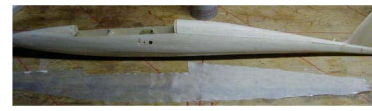
As the resin soaks into the wood, it creates a rigid skin. The glass, when bumps & any puckers are sanded down & a "flow coat" of thinned resin applied to wet sand glass smooth, makes a good surface for filler, primer & paint. Optionally, when the single layers are on & cured enough to sand the overlaps smooth, an additional layer may be applied over the bottom to help reduce dings from landings. Let fully cure, feather edges & apply the flow coat, etc. as detailed in File 1.
