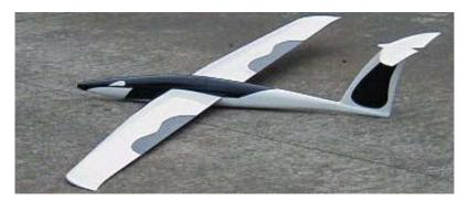
This original version had 1" TE sweep shown here. It looked racy, but areas ahead & behind the pivot rod were substantially dissimilar which made hard work for servos at higher speeds.
