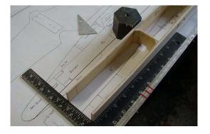
Butt the front ends to the inside of a carpenter's square so they are <u>perfectly</u> aligned in top view. Press flush to the workbench so sides are aligned in profile. As shown in the next pic, TS can be glued to the edges of the sides before joining them to the formers, but leave a little space to fill in next to the TS on the formers on the unattached side.
