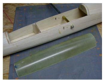
Note holes & slots made for the pitcheron hardware. Trim the canopy (Harley's pack) to the inside edges of its exterior molded-in reference lines. If too wide or too narrow, use a heat gun to make it pliable. To widen, press it down with a thick glove. To narrow, squeeze between strips of wood tacked to a board. Mark inside canopy ends to outline the  $\frac{1}{4}$ " plates it rests on. Tape it in place to merge top fuselage contours to it.
